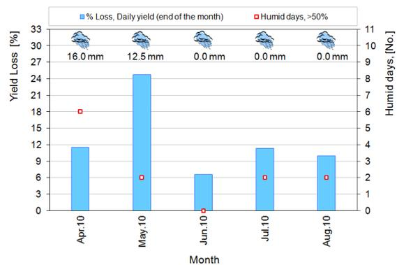
**Figure 4:** End of the month percentage loss in daily yield due to dust accumulation.
